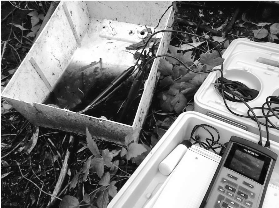
Figure 1. Small illegal anthrotelma with a Multi 3401i (WTW).
