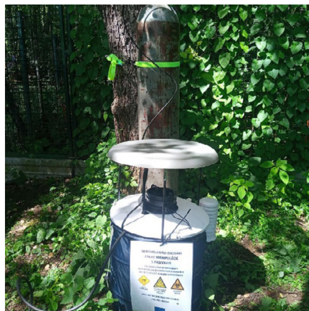
Figure 1. Photograph of BG-Sentinel 2 traps (Biogents, Germany) from Zoo Košice (Grundmann et al. 2025).
